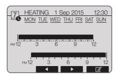
Hours of the day are shown as a bar across the main part of the screen. Where the bar is solid black, heating/DHW (whichever is selected) is allowed.
